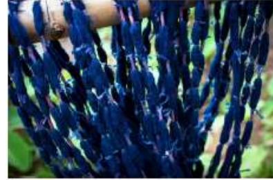
The thread with tied pattern is dyed to obtain the desired pattern
