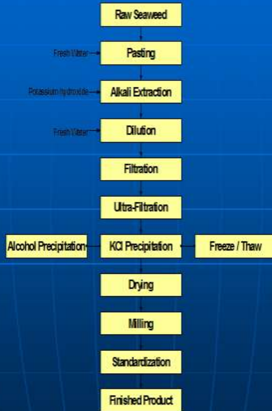
Picture 4. Manufacturing Process of Refined Carrageenan
