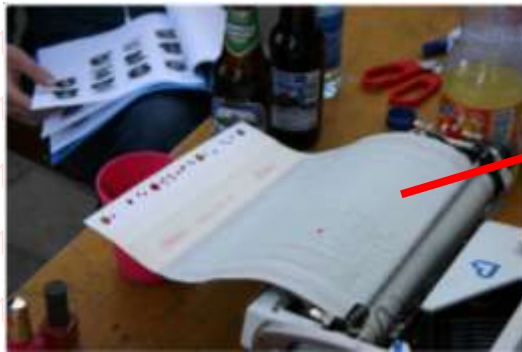
Forming letters on stencil using typewriter
