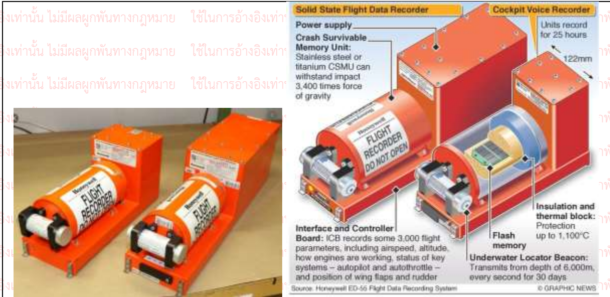
Picture 1. Actual photo of FDR and CVR and their components
