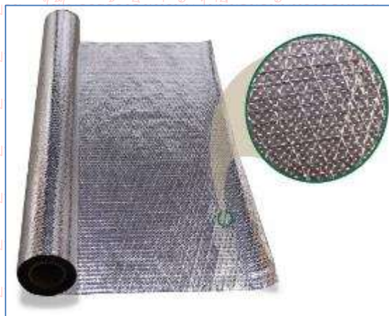
Two-sided reflective aluminized polyester film with reinforced scrim inside, designed to reflect radiant heat. Weight 16.35 lbs per 1000 sq ft roll. Thermal Properties : Emissivity: 0.05, Reflectivity: 95%, Standard: ASTM C1371-04a
