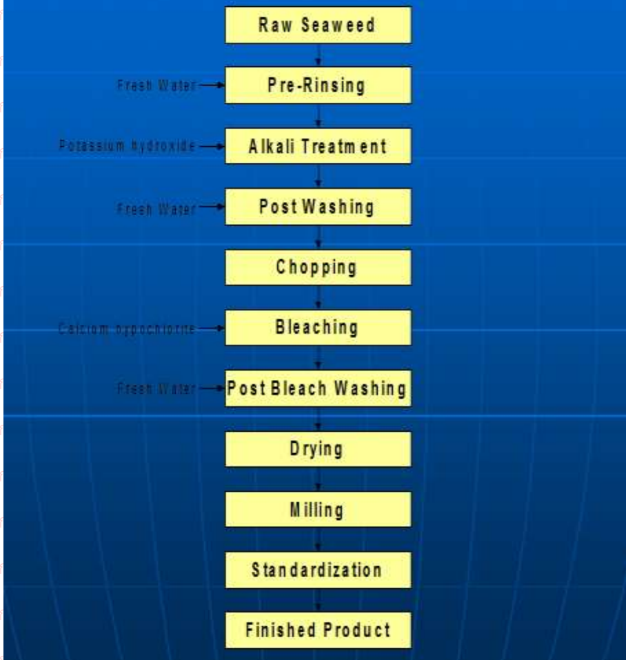
Picture 3. Manufacturing Process of Semi-Refined Carrageenan
