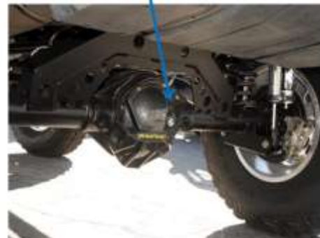
Rear axle housing (consist of crown wheel and pinion)
