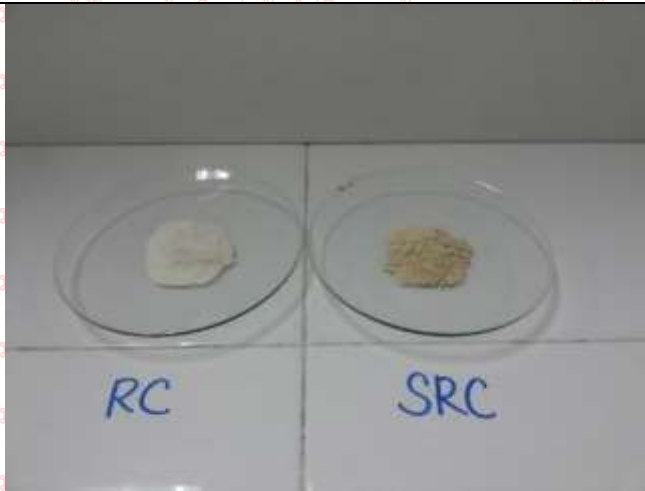
Picture 1. Refined Carrageenan (RC) and Semi-Refined Carrageenan (SRC) Powder In powder form, RC is whiter than SRC
