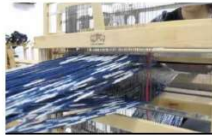
The dyed thread then weaves to make into a finished fabric
